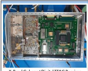
X-Band Coherent Digital TT&C Receiver
