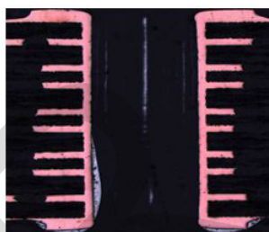
PTH shows better Electroless copper integrity a. after 6X solder float test and b. thermal cycling test
