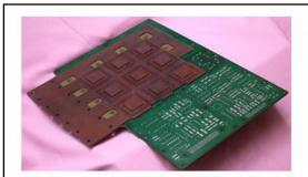
Copper bonded Metal core
