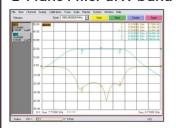
Measured Response of X band filter
