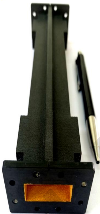
Black color novel anodic coating on waveguide
