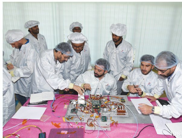
UNNATI Batch-1 participants integrating the nanosatellite
