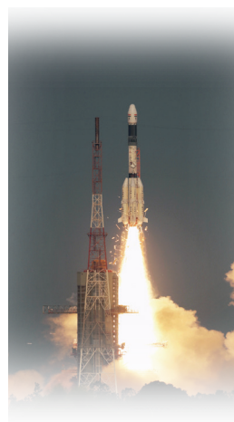
Launch of GSAT-6A by GSLV-F08 with indigenous cryogenic upper stage (March 29, 2018)
